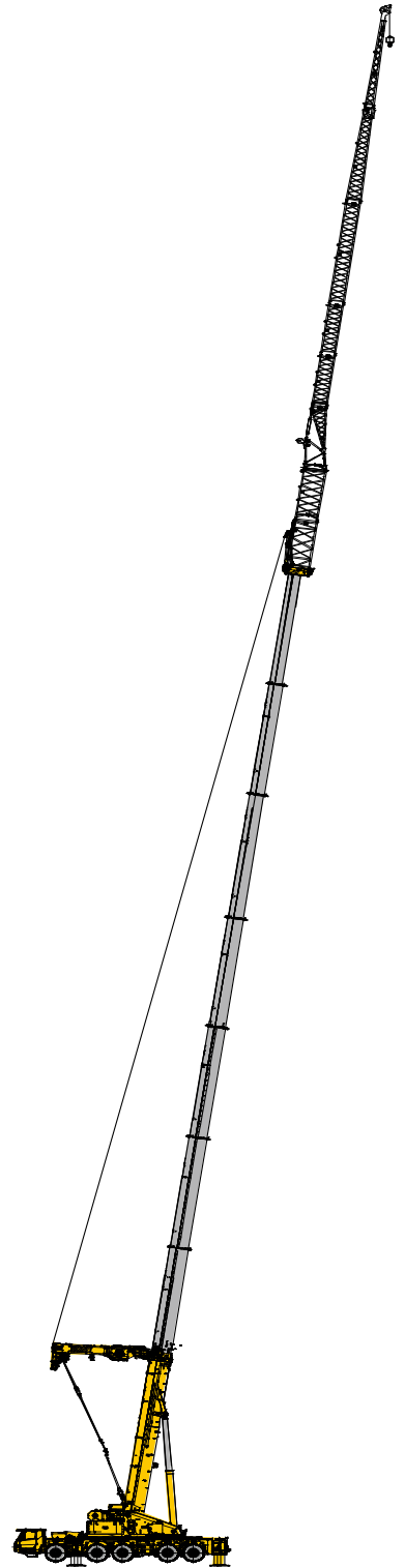
超起+固定副臂 Super lifting device + fixed Jib
